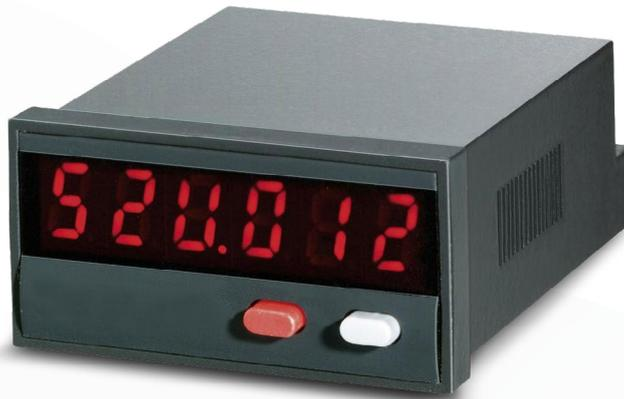
**The 52UK.2 is a voltage-powered dual function counter with 4 functions in one device: counter with 2 totalizing ranges; totalizer and timer; totalizer and frequency meter; timer with 2 time ranges. For fast and slow count pulses, with 6-digit LED display for NPN, PNP input signals.**
